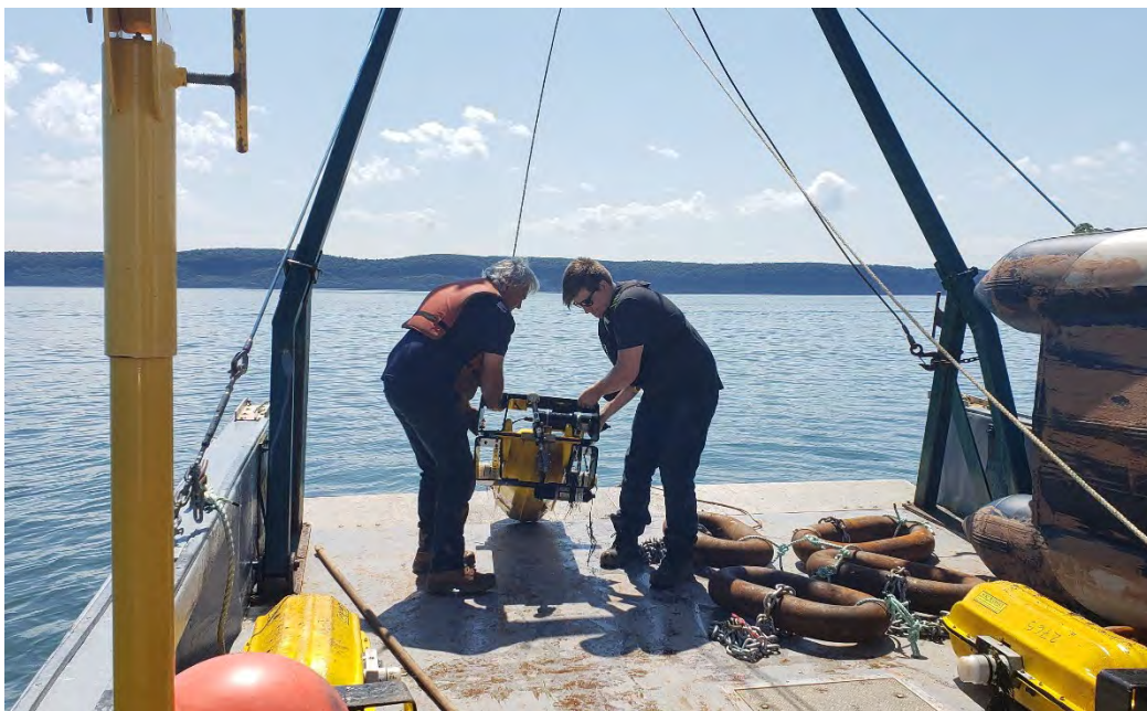
Figure 4. C-PODs: Ocean technology staff haul a C-POD SUBS package aboard during recovery.
