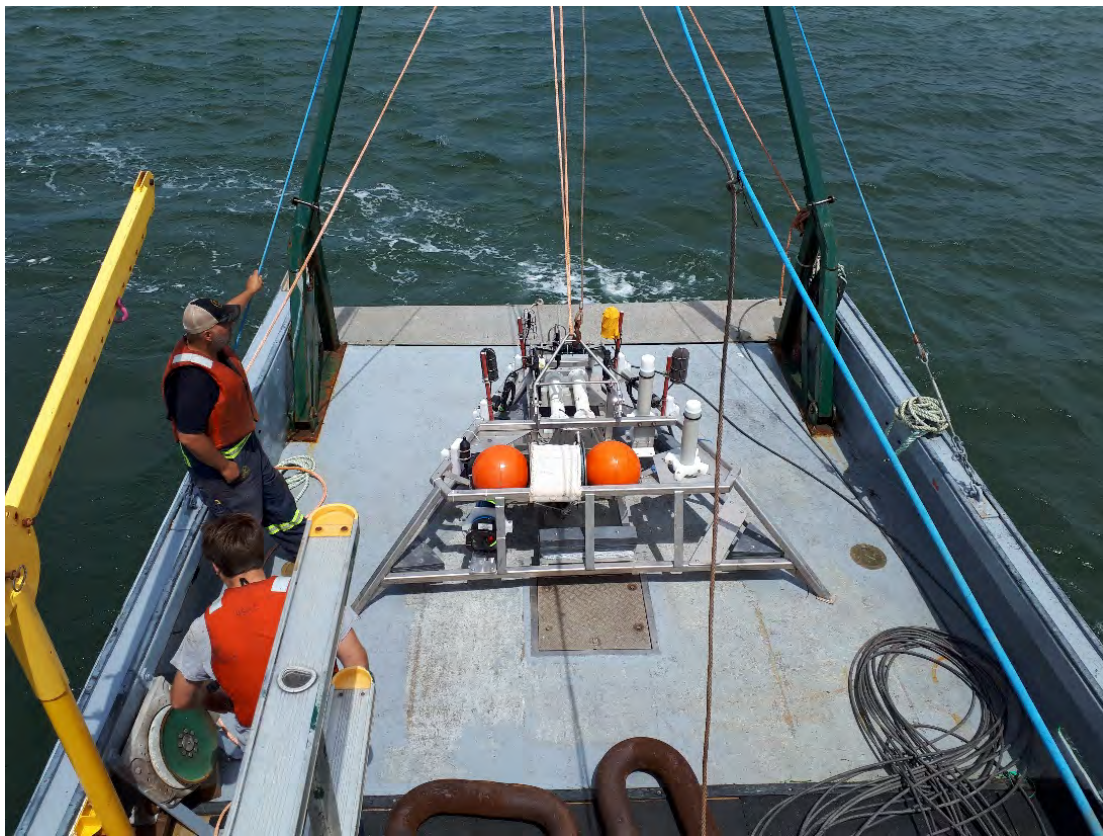
Figure 8: Five PAM devices were mounted on the FAST platform for the comparative PAM study. Photograph depicts the platform on the deck of the Nova Endeavour prior to deployment at the FORCE site.
